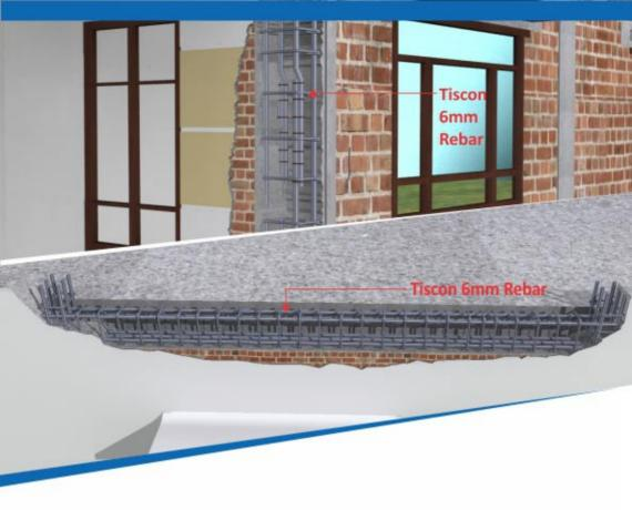
IS 456: 2000 specifies conditions for providing 'minimum reinforcement' to various structural members. Sections 26.5.1.6 (beam stirrups) and 26.5.3.2 (column reinforcement) clearly allow for 6mm stirrups\* to be used at lower steel intensity.
