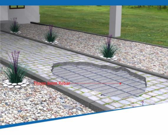
Pavements and hardstanding, which require 'nominal reinforcement', are better and economically detailed with Tiscon 6mm rebars. This application is not limited to your house but beyond at public places as well, if conditions are appropriate.
