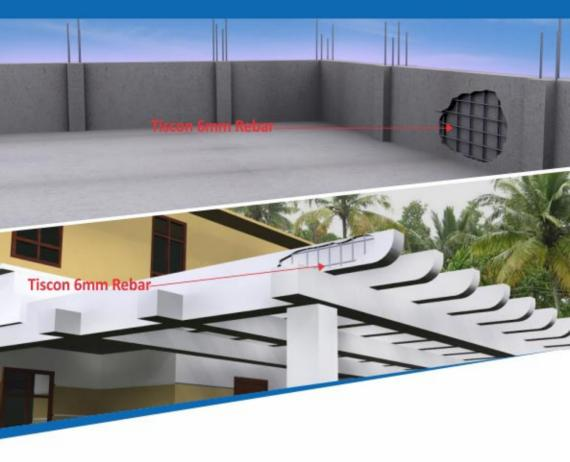
Many of the structurally not so- critical elements could use 6mm rebars to take care of 'nominal reinforcement' requirement. RCC parapet walls, facia and other facade elements could be detailed with a mix of 6mm and 8mm rebars.
