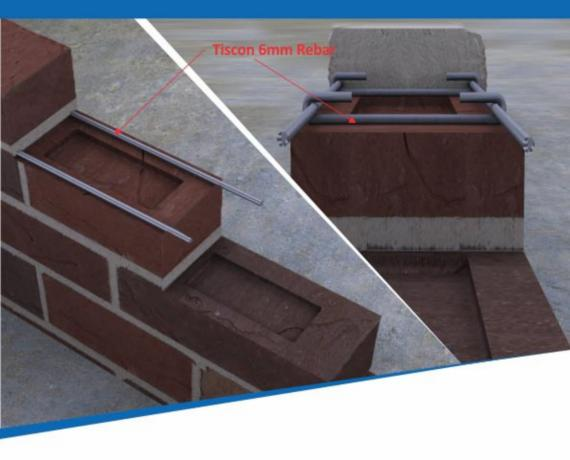
Masonry Reinforcement improves the structural performance of masonry walls by providing additional resistance to lateral loads e.g. wind. It also reduces the risk of cracking either at stress concentrations around openings or as a result of movement. 6mm rebars are used in masonry reinforcement to provide a definite structure to the wall. Concrete bands as shown above, are used to improve response of brick- masonry units during earthquakes.
